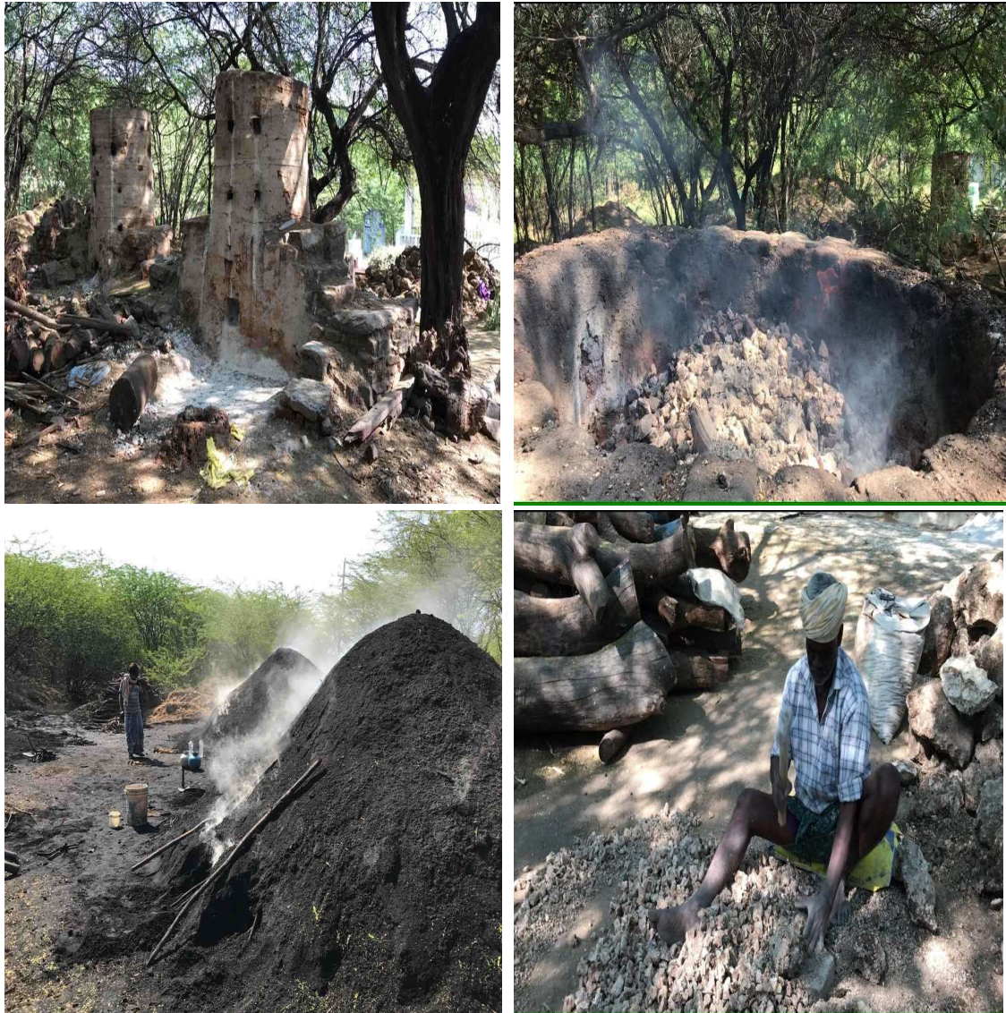
1Clockwise from Top Left: 1. Limestone kilns; 2. A charging kiln from a top view; 3. A laborer cutting large raw limestone into small pieces for kiln charging; 4. Charcoal is prepared nearby as fuel for the kiln. Limestone kilns are still in operation for quicklime production, used for domestic and agricultural purposes. These images were captured at Dodderi near Chalakere as a representation.
