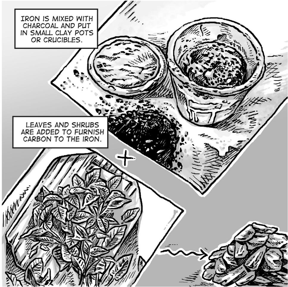
IRON IS MIXED WITH CHARCOAL AND PUT IN SMALL CLAY POTS OR CRUCIBLES.
